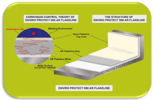
This product can be used both on metal and concrete surfaces. Both surfaces shall be blasted and cleaned. Although concrete surfaces require primer, metal surfaces do not require primer
